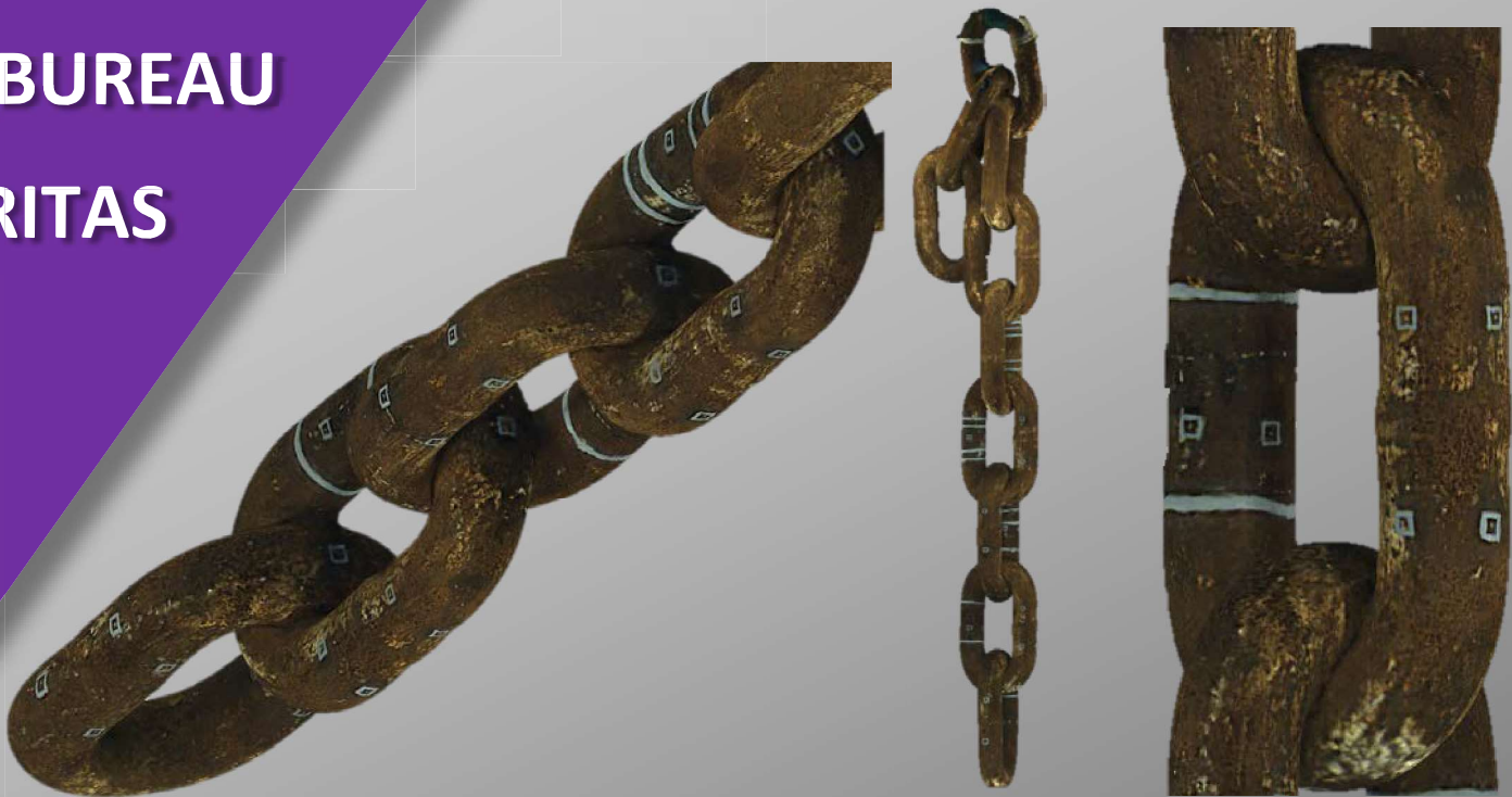
3D models of 90mm mooring chain - Generated by ORUS 3D
