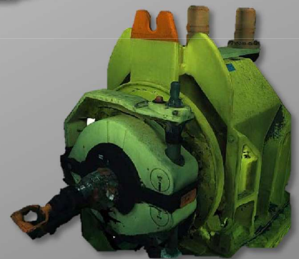
3D models of Damaged Spool pieces and Jumper metrology Generated by ORUS 3D
