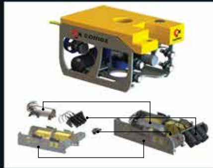
System skid with adapted buoyancy
